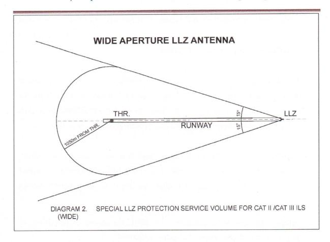
**Note:** ICAO Annex- 10 Volume-I Radio Navigational aids, Attachment C, defines the Aperture of Localizer antenna as follows:
